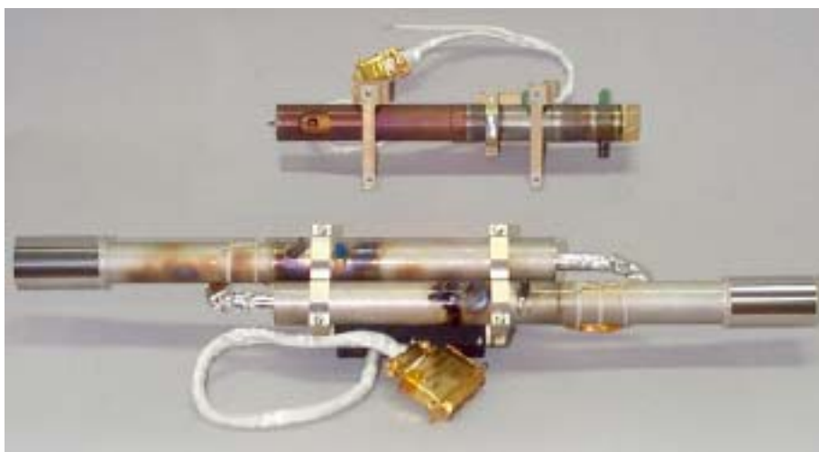
Figure 13. The PIA photometers with PIA-3 at the top, and the PIA-1/2 assembly below.
