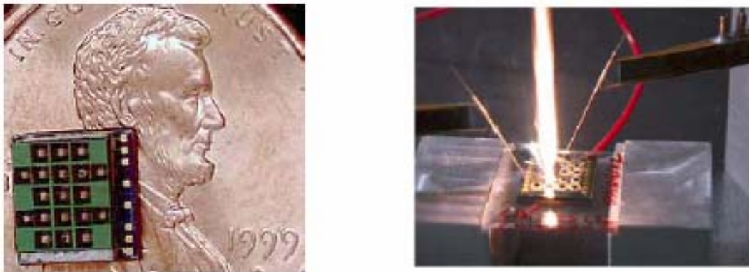
Figure 5. Left: 3x5 microthruster array 'Rocket Chip'. Right: Firing a microthruster (C. Rossi, LAAS-CNRS)
