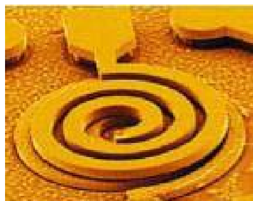
Figure 3. Examples of MEMS low loss inductors: left: Yoon, Chen, Allen & Laskar, Georgia Tech, right: "Above IC technology", MEMSCAP Transducers 2001
