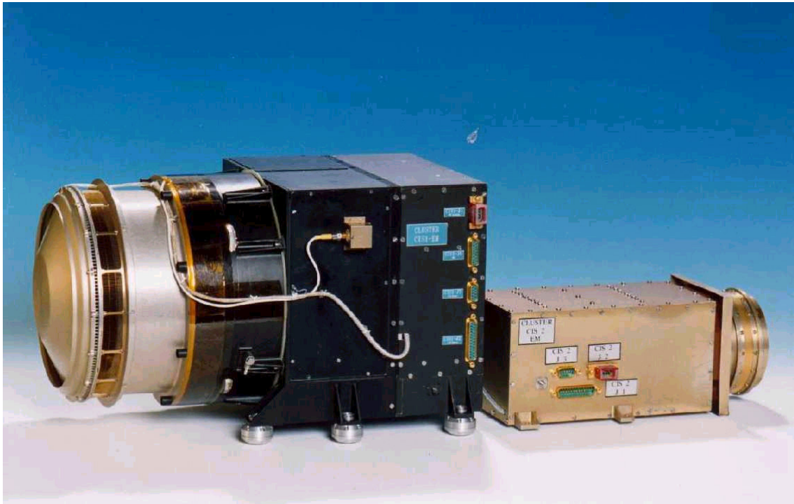
Figure 3.2.1 The CODIF (on the left) and the HIA (on the right) ion detectors of the CIS experiment
