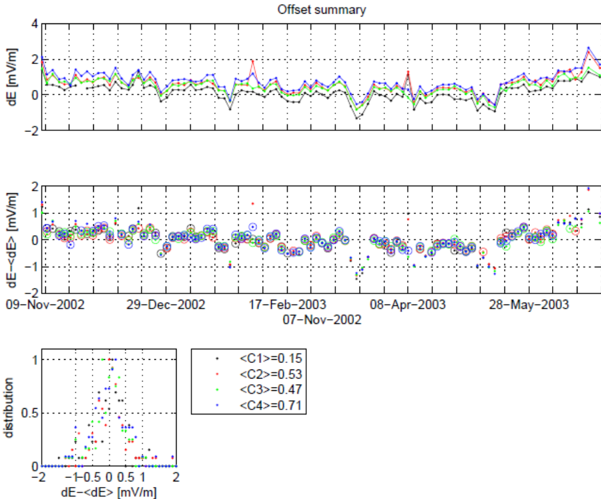
Figure 18: ISR2 offset summary ( E_x ) in the SW/MSH for spring 2003. The top panel shows the instantaneous offsets determined for each orbit. The middle panel shown the difference between the instantaneous offsets and the average “seasonal” offset which is used in the CAA production ( \langle C1 \rangle.. \langle C4 \rangle in the panel below), and which is computed on the basis of the encircled points. The distribution of the difference if shown in the bottom-left panel.
